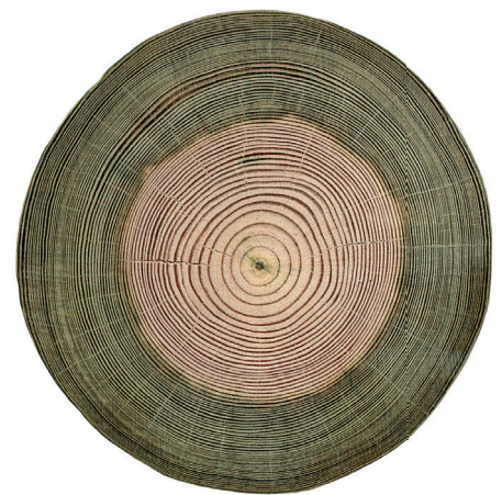
Pinewood pole impregnated with Korasit® KS2: Even penetration in the entire sapwood area (impregnable zone).
